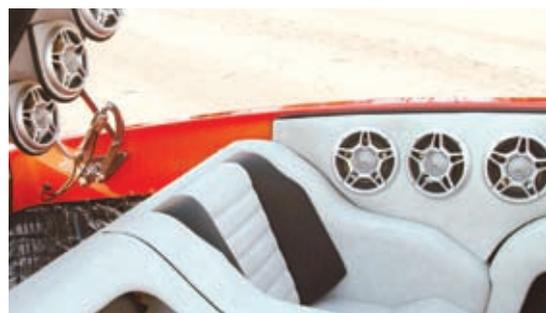
compatible computer with 10.1-inch touch-panel screen, and the rest of the 'dash' features four pairs of Arc's Kar 265 6.5-inch component sets, while down lower, where kick panels would go, are eight Arc 8-inch Dual VC woofers. Two more 15-inch subs pound out the bass when the boat is cruising on the open water.
