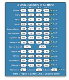
Into 4-0hm non-inductive loads the 4200 SE produced an average output of 124.75 Watts at 1% THD, exceeding the manufacturer's specification by 13.5%. Overall, the 4200 SE spec'd out very well (into 4-0hm loads) in the majority of our measurements.
