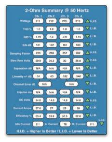
The 4200 SE also exceeded manufacturer specifications into 2-0hm non-inductive loads by an average of 7.25%. This amplifier has also established itself as being stable and linear into half-loads, doubling its power from 4-0hms to 2-0hms, as promised by ARC Audio. Traditionally, most amplifiers weaken significantly, as nominal resistive loads fall below 4-0hms; however, the 4200 SE retained its composure, varying ever so slightly in performance and in some instances, actually improved.
