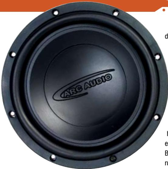
for a little less efficiency but more low frequency output. In terms of a vented application, Arc Audio suggests a 0.6 cubic foot enclosure with a 2-inch ID vent with a length of 12 inches. This tunes the enclosure to 34Hz and was the one I decided to go with. Long-time friend Mark Feeney at Sell Thru Displays custom build the enclosure for me and I took care of the speaker cutout and vent back at the test lab.
