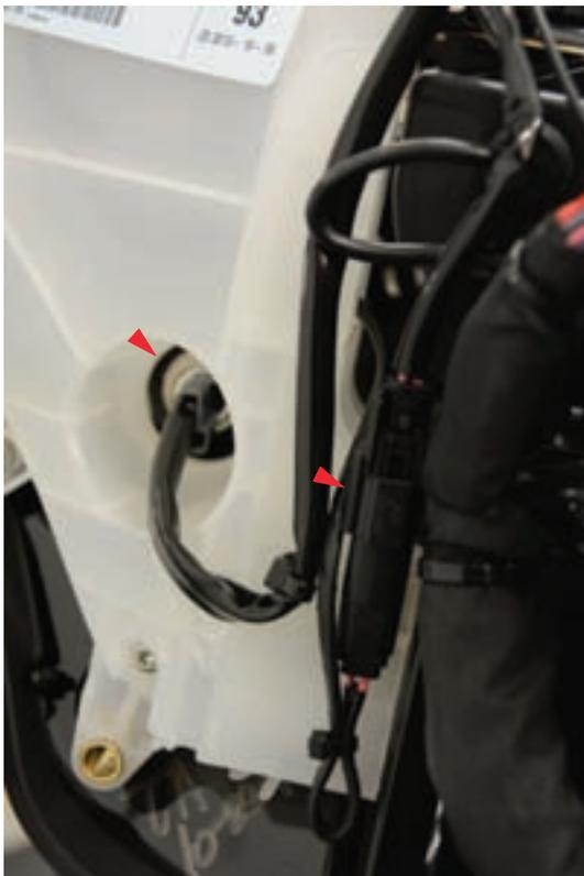
14. Disconnect speaker wiring harness and pop its fastener free from the enclosure. On the right hand side you will need to pull the power port (cigarette lighter) harness off the power port.
