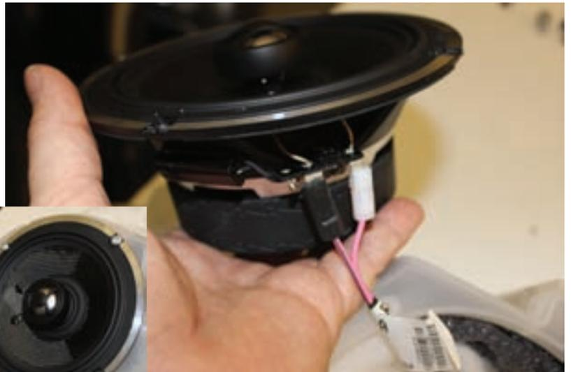
Mount the speakers using the original hardware. Be careful not to over tighten the screws.
