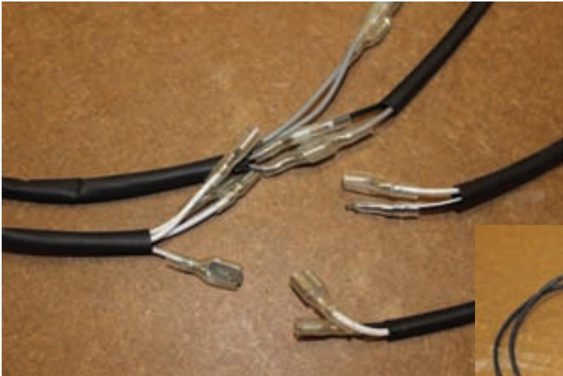
21. You now need to assemble the speaker harness. Just plug the adapters to the ends of the harness, matching the connectors with their appropriate mate and wire color. Make sure the insulating covers are firmly in place. A shorted wire here will shut down or possibly damage the system.
