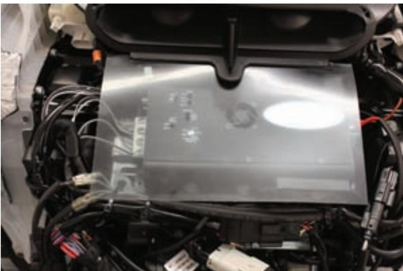
29. This is what it should look like when it's done. Tie up all the extra wire using the supplied zip ties and reverse the process of disassembly. Everything should do together easily without any need to excessive force. Time to fire it up and listen to it.
