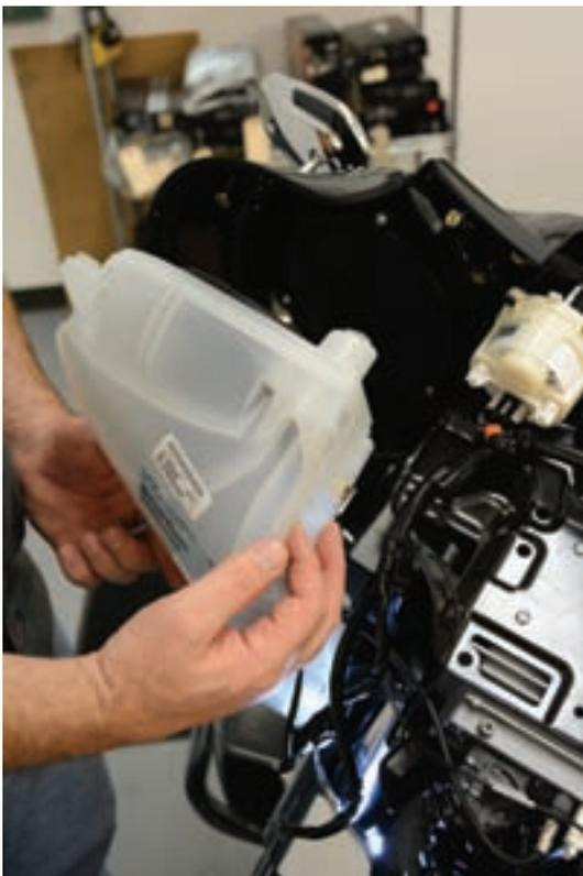
The enclosure should be loose and come off freely. If the enclosure does not come off easily don't force it, repeat these steps and insure you have fully removed all fasteners.
