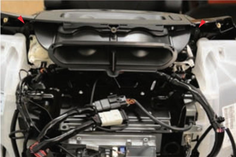
15. Remove the 2- T25 Torx head screws that retain the vent assembly and remove it by pulling it forward.
