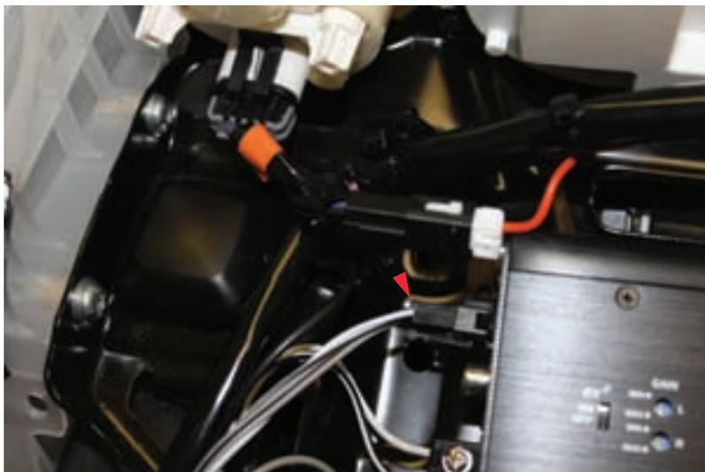
26. Connect the black 5 pin plug to its mate on the end of the amplifier next to the RCA connectors.
