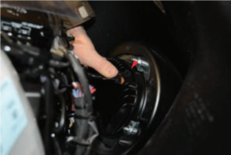
12. Gently pull the outer fair toward you. You will need to lean over the fairing and locate the headlight wiring harness. Disconnect the headlight harness and let it hang. If no aftermarket accessories have been added, you can now remove the fairing. Set it in a safe, out of the way location where it will not be dropped or damaged
