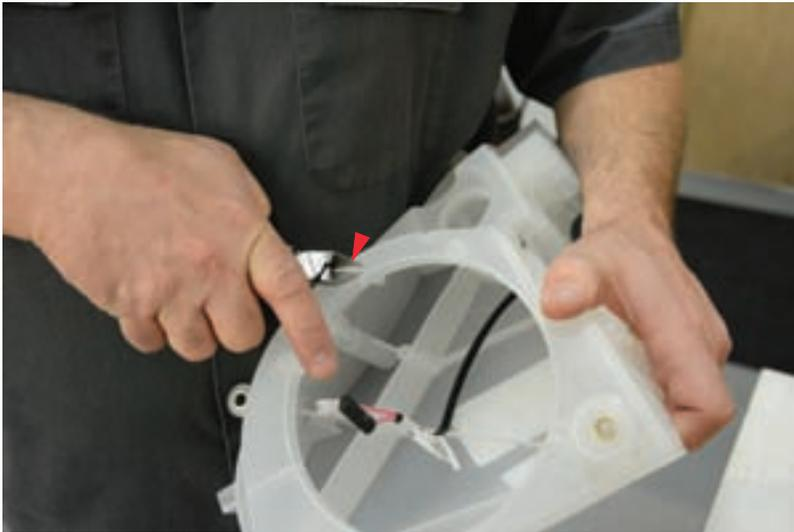
19. After removing the stock speakers, trim any alignment pins on the mounting surface flush with the face of the enclosure.
