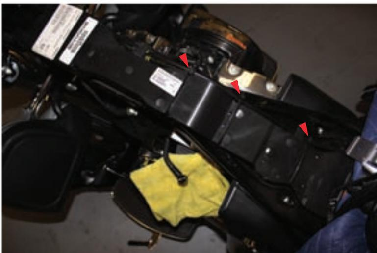
Special Note: This 2014 model has had 3 zip ties added under the tank the secure the brake lines. If your bike does not have these it is recommended that you contact your local dealer and find out if it is necessary. If they are present they must be replaced exactly as they are. ARC Audio takes no responsibility for this modification.
