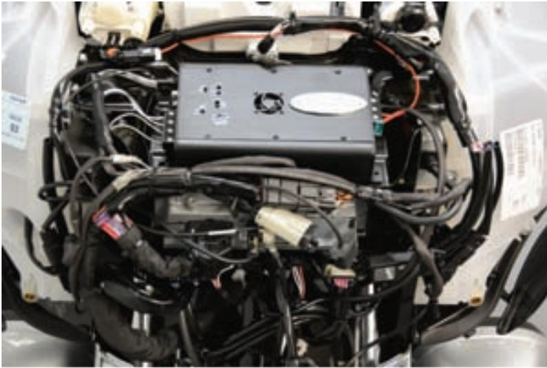
24. Attach the amplifier to the top of the amplifier bracket using the large Velcro pad. You only get 1 shot with this stuff so be careful.
