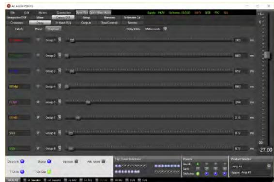
Output Signal Delay (Up to 30msPper Channel)
