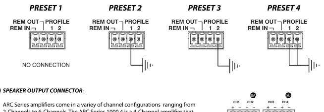
2-Channels to 6-Channels. The ARC Series 1000.4 is a 4-Channel amplifier that produces up 250 Watts RMS per channel at 2-Ohms or 4-Ohms. Each pair of channels may also be bridged at 4-Ohms making the ARC 1000.4 a very powerful 2-Channel amplifier.
