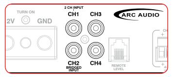
recommended that you use an appropriate RCA cable with one set of ends removed as inputs for the amplifier.
