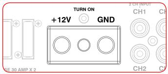
The Turn On input should be connected to the amplifier +12V DC remote turn-on output of your after-market source unit. In most cases this is a blue wire with a white stripe. Note: On some source units, there are power antenna AND remote turn-on wires. If you only hear audio when listening to the AM/FM tuner, your amp may connected to the wrong wire.
