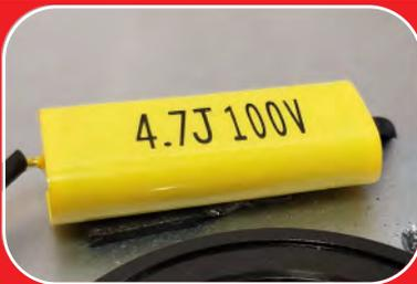
*An high-quality passive crossover is integrated into the rear magnet cover housing. The filter prevents low-frequency information from damaging the HLCD diaphragm. The result is crystal-clear sound and incredible power handling.*
