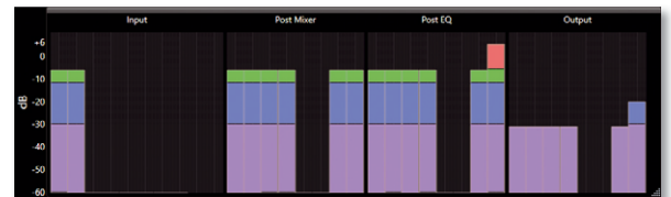
A nice goodie: The VU meter shows the levels at the inputs, before and after the EQ and at the outputs
