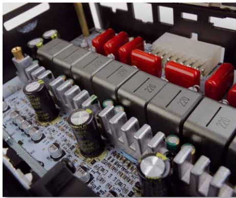
The four amplifier ICs are screwed to the housing with a ribbed heatsink strip
